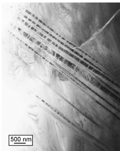
Fig. 3.5-8: Bright-field TEM image of quartz shock-loaded to 23 GPa containing abundant PDF lamellae with {11.2} orientation.
