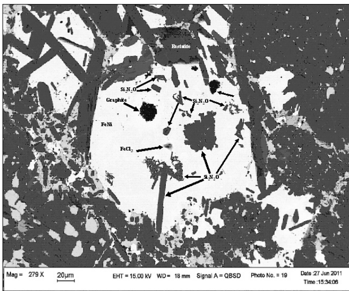
Fig. 3.2-6: An FeNi metal nodule containing inclusions of three early condensate assemblages: sinoite- and oldhamite-bearing fragments, sinoite-and oldhamite-bearing graphite and lawrencite.
