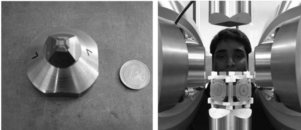
Fig. 3.6-4: (left) Composite anvil with a tungsten carbide core that is supported by a steel jacket. (right) Six second stage composite anvils are guided by an aluminium cage and compressed by large first stage anvils.
