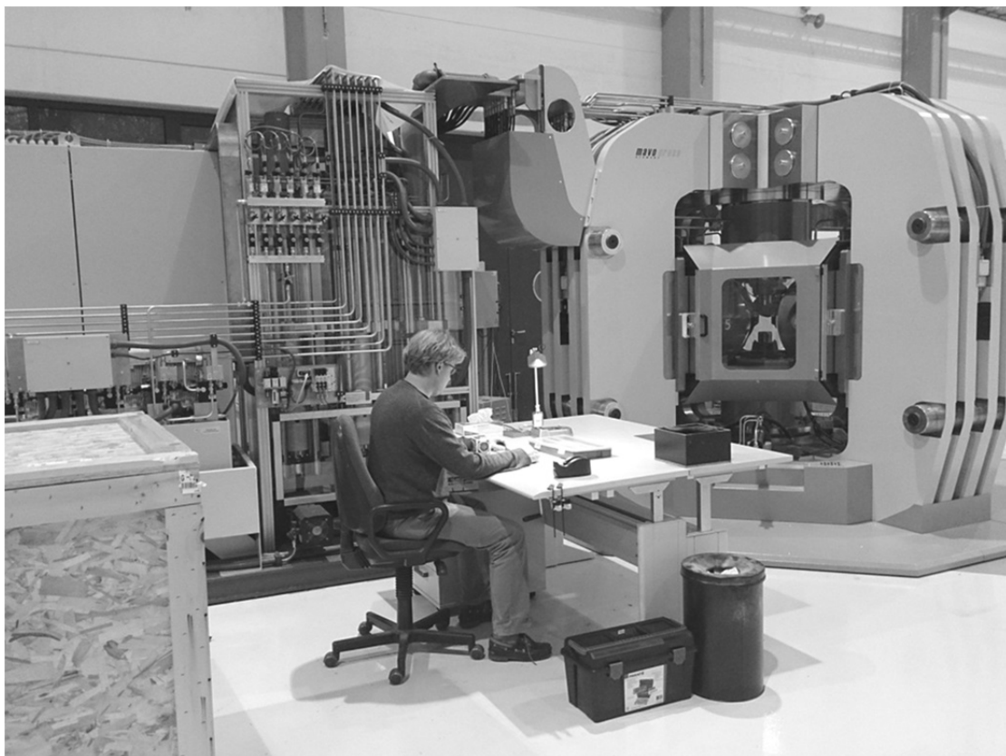
Fig. 3.8-4: The SAPHiR instrument at FRM II in Garching. The large wooden case on the left contains the recently delivered 640 position-sensitive ^3\text{He} detector tubes. The future neutron beam will come from the right.
